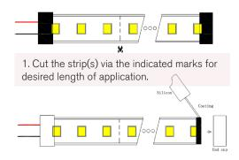
2) Apply silicone caulk on cut end and attach end cap. Wait 30 minutes for silicone to solidify.
